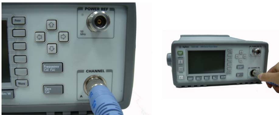
Figure 1-2 Connecting a sensor cable to power meter
