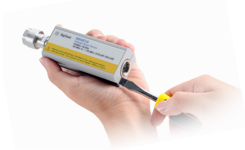
Figure 3-2 Removing power sensor shell
